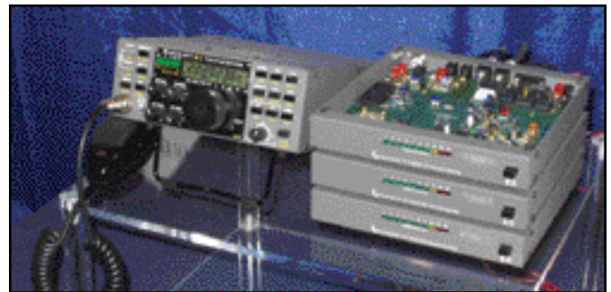
Elecraft's transverters for 6 meters, 2 meters, and 222 MHz will put your K2 or any other HF rig on VHF SSB and CW.
