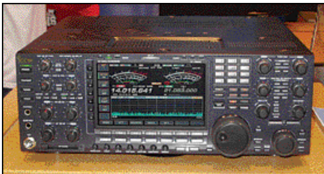
ICOM's new IC-7800 is a top-of-the-line HF+6-meter transceiver designed for fixed-station use.
