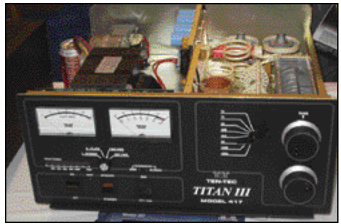
The Ten-Tec Titan III amplifier runs 1500 watts PEP on all amateur bands between 160 and 15 meters (except 60 meters), and can be modified to operate on 12 and 10 meters if you have proof you're a licensed ham.
